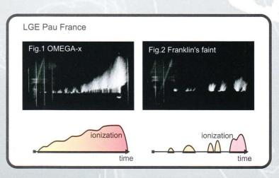
In Franklin's traditional faint, the triggering of the upward leader occurs later than in the OMEGA-x. This is caused by a longer than in OMEGA-x initial transient state, during which leaders are generated and instantly fade away as a result of forming of the electrical discharge around the tip (Fig.2).
